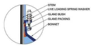
**Metal Seated Valves** - The key advantage of metal seated valves when compared to soft seated valves is that they can withstand high temperatures and severe service conditions. Metal seats can stand up to extreme flashing, hydraulic shock, abrasive process fluid, and high temperatures up to and exceeding 1,000° F. They are also ideal for high erosion or corrosion applications. Another important factor is that metal seats can be hardened by specialized coatings.
