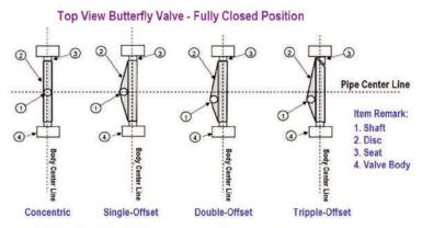
Single-Offset - The shaft is offset from its body center line.
